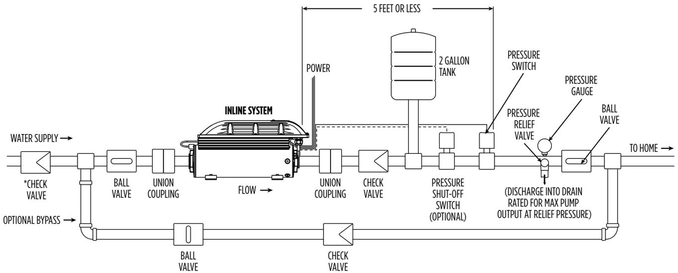
*NOTE: These optional components are shown in a typical installation diagram. They should be used at the installer's discretion as required for particular applications.
